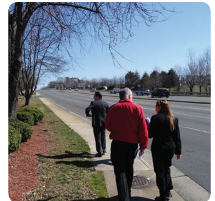
Narrow sidewalks without a buffer from traffic
